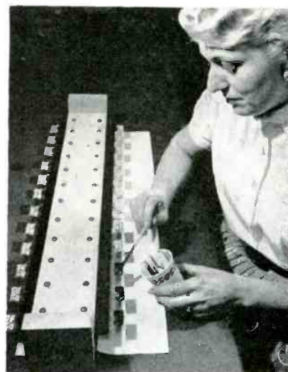
Applying epoxy resin coating to finished amplifiers with wood paddle, using 24-unit turnover holding fixture
