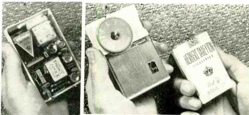
Japanese pocket radio manufactured by Tokyo Tsushin Kogyo uses five transistors, one diode and a 2¼-inch dynamic loudspeaker, operates from a 22.5-volt battery. The set has a sensitivity of approximately 1 mv/m and weighs 290 grams
