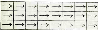
Figure 2—Magnetized material (domains rotated into alignment)
