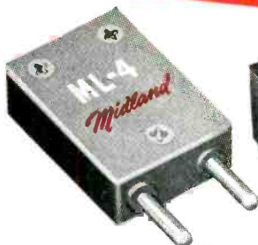
Type ML-4. Range: 2.0 mc–10.0 mc. Supplied per mil Type CR-5, CR-6, CR-8, CR-10 when specified. Holder is phenolic, gasket sealed. Pin diameter: .093 \pm .002 Pin length: .400 \pm .030
