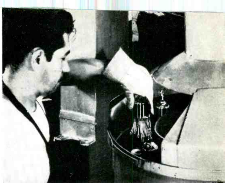
Wire-stripping tank uses Lonco chemical stripper to remove insulation. Ends of leads are suspended in liquid for one revolution around doughnut-shaped pan filled with stripping chemical
