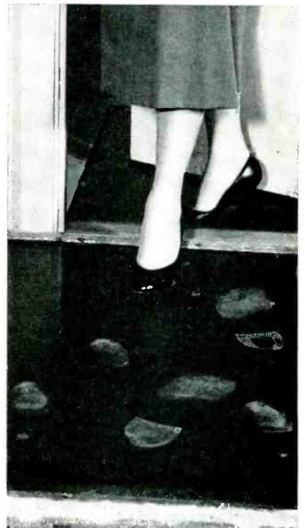
Gelatin mat at entrance to White Room used for transistor research shows relative amounts of dust removed from men's and women's shoes
