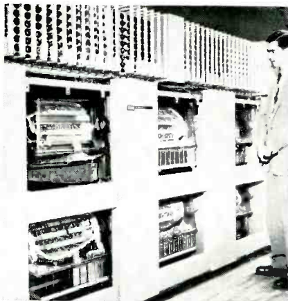
Twenty-four magnetic drums provide high speed buffer storage. Drums rotate at 3,000 cps and store 500,000 bits each
