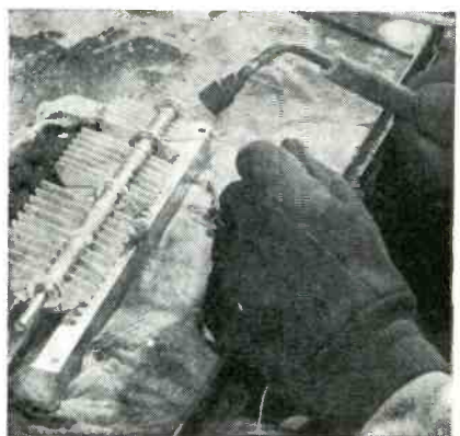
Soldering coin silver disks and rotor plates with gas torch after swaging
