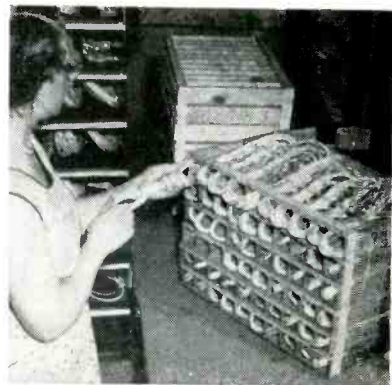
Loading all wires for a particular harness in kit box having numbered bins
