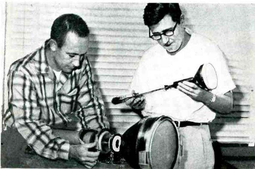
Novel cathode-ray tube being examined by I. W. Fuller, Jr. of NRL was developed by Sylvania for the Navy. The screen diameter is 5 inches. Larger tube in experimental radar circuit is inspected by N. L. Davis
