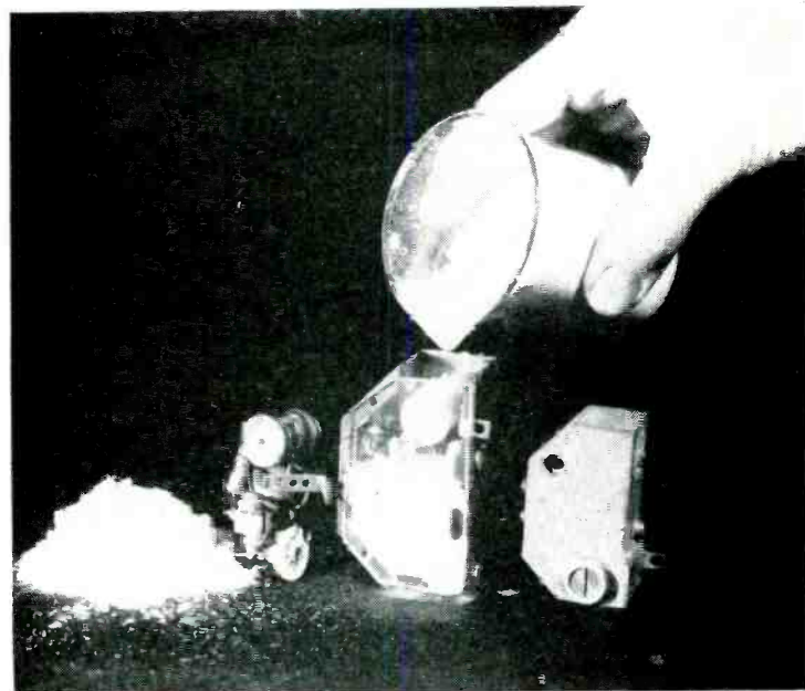
One-tube assembly before and after encapsulation with Eccofoam GL phenolic-epoxy powder (Emerson & Cuming; that foams when heated). Socket is flush with rear side of embedment. For temperatures up to 600 F, same firm's Stycast 2662 epoxy resin is used instead
