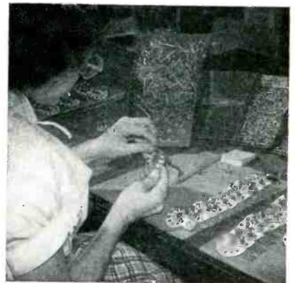
Work setup for inserting coils in tuner wafer
