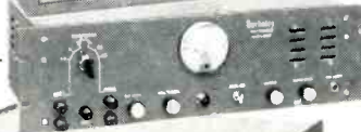
Model 5590 WWV receiver permits calibration of 5571 within \pm 2 parts in 10^5 , for use as secondary frequency and time standard. Price, $495.00
