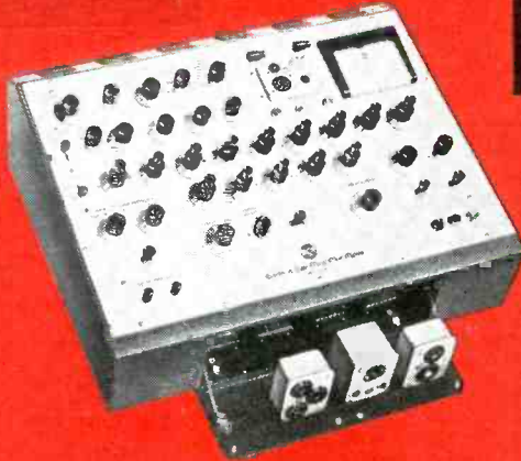
ELECTRON-TUBE M. CROMHOMETER — WT-100A Versatile tube tester with accuracy approaching that of tube-factory equipment for measuring true g_m . Has many operational features especially suited for electronics equipment manufacturers, research and development, and maintenance groups... anyone desiring to test tubes under actual voltage and current conditions.
