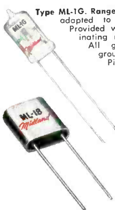
Type ML-18. Range: 5.0 mc–150.0 mc. This unit is a metal counterpart of the ML-1G. Hermetically sealed holder with glass and metal base. Available with fixed pins if desired instead of the wire leads illustrated here. Pin diameter: .040 \pm .002 Pin length: .234 \pm .030 Wire: .017 \pm .001 Dia. by 1.500 \pm .062 long
