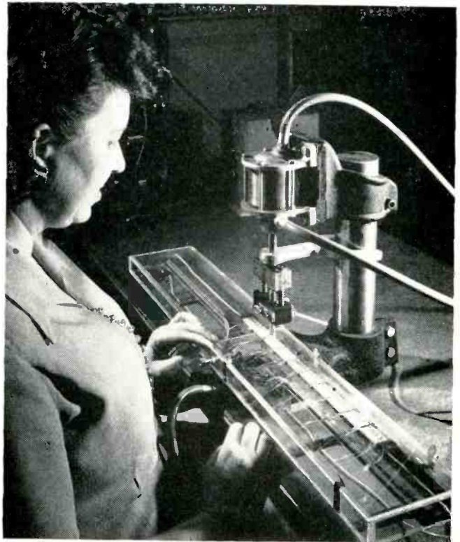
Air-operated soldering iron hermetically seals transistors in cavities of blocks under accurately controlled atmosphere of dry air
