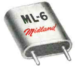
Type ML-6. Range: 1.0 mc–125.0 mc. Supplied per mil Type CR-18, CR-19, CR-23, CR-27, CR-28, CR-32, CR-52, CR-54, CR-33, CR-35, CR-36, CR-48 when specified. Hermetically sealed metal holder with glass and metal base. Pin diameter: .050 \pm .002 Pin length: .238 + .010 - .015
