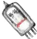
Type ML-2G. Range: 200 Kc–150.0 mc. An all glass 7-pin miniature of the same dimensional proportions as the 2AK5 miniature receiving tube. Pin diameter: .040 \pm .002 Pin length: .250 \pm .030
