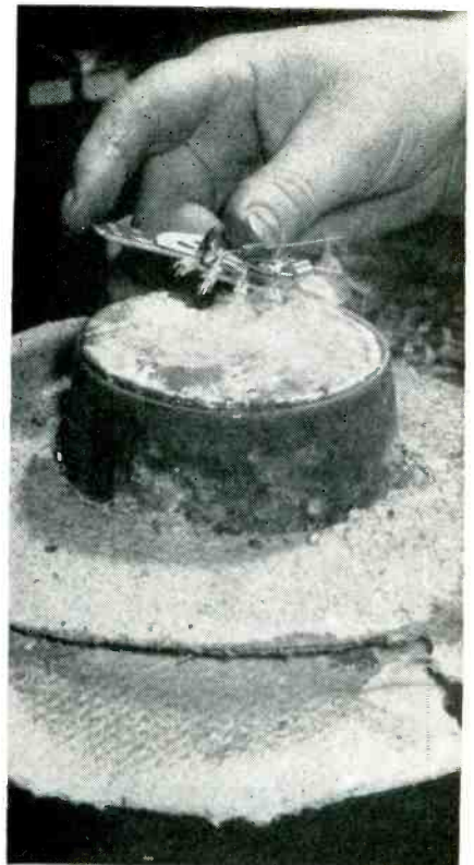
Holding wafer assembly over curved indentation in rim of special solder pot, in readiness for dip-soldering of terminals
