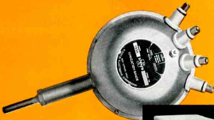
Ionization Gauge and Amplifier cover 10^{-4} to 10^{-7} mm Hg.
