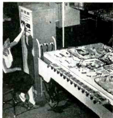
Automatic hi-pot and continuity checker being used for final test of finished harness on special board, to reduce testing time from 40 hours to about 40 minutes for average harness. Unit stops when defective wire is reached
