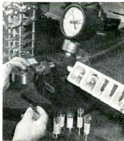
Matching bearings to bearing holes within 0.0002 inch with comparison air gage operating at 34 lb air pressure
