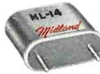
Type ML-14. Range: 3.0 mc–75.0 mc. Identical in performance to Type ML-6 except for height of the metal can. Pin diameter: .050 \pm .002 Pin length: .238 + .010 - .015
