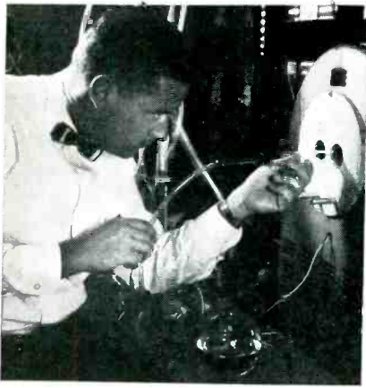
Engineer prepares germanium blanks for new surface-barrier diffused transistors. Tiny boats in the quartz tube carry bits of germanium while gas flowing through the tube, as it rests in the furnace, contains particles of metal which diffuse into the surfaces of the germanium blanks. The technique includes etching to give
