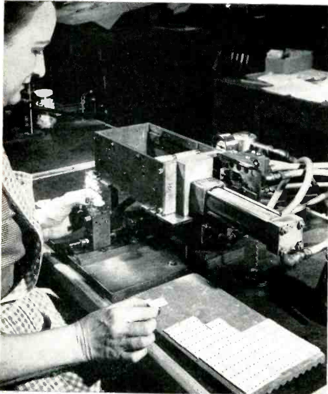
Setup for screen-printing silver conductors and carbon resistors on steatite blocks that serve as amplifier chassis
