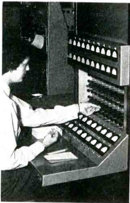
Conveyorized burning-in test set, with operator inserting transistor leads in socket on endlessly moving belt
