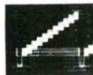
STAIRSTEP SIGNAL modulated by crystal controlled 3.579 mc for differential amplitude and differential phase measurement. Checks amplitude linearity, differential amplitude linearity and differential phase of any unit or system. Model 1003-C includes variable duty cycle stairstep (10-90% average picture level).
