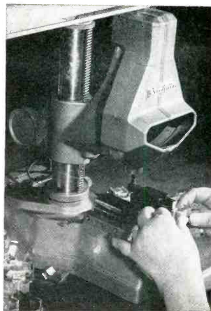
Method of using gage to check average thickness of individual silver-plated plates in assembled stator
