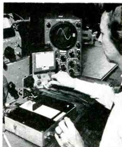
Final test station for finished transistor amplifiers. Operator pushes seven leads down between plastic wedges into contact blades to make all connections simultaneously for gain, frequency response and noise tests
