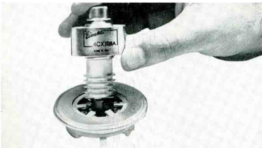
Ceramic power tetrode is forced air-cooled and fits into special socket designed for new type construction
