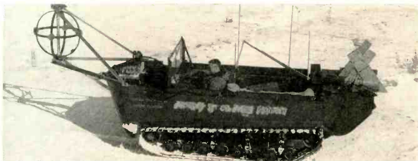
Army weasel equipped with General Mills-designed loop antenna system is used to test new trail marking system on the ice cap of Greenland
