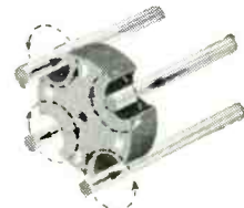
Figure 7—Conductor arrangement for multi-pole magnet
