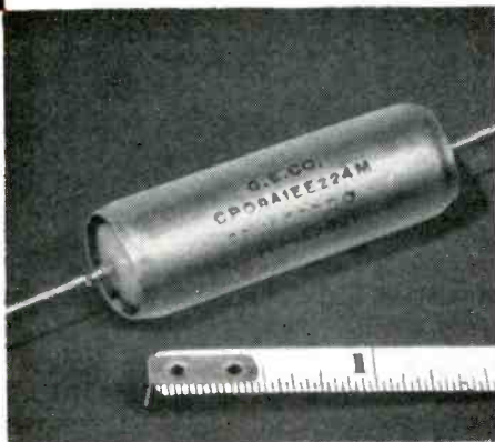
METAL-CLAD TUBULAR CAPACITORS — +85C, mineral oil impregnated. Built to MIL-C-25A. Ratings: .001 to 1.0 uf, 100-600 v. d-c. Tol: \pm 5\% , \pm 10\% , or \pm 20\% . Write for GEC-1390.
