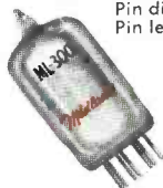
Type ML-18. Range: 5.0 mc–150.0 mc. This unit is a metal counterpart of the ML-1G. Hermetically sealed holder with glass and metal base. Available with fixed pins if desired instead of the wire leads illustrated here. Pin diameter: .040 \pm .002 Pin length: .234 \pm .030 Wire: .017 \pm .001 Dia. by 1.500 \pm .062 long
