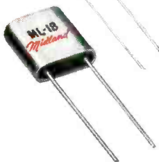
Type ML-18. Range: 5.0 mc–150.0 mc. This unit is a metal counterpart of the ML-1G. Hermetically sealed holder with glass and metal base. Available with fixed pins if desired instead of the wire leads illustrated here. Pin diameter: .040 \pm .002 Pin length: .234 \pm .030 Wire: .017 \pm .001 Dia. by 1.500 \pm .062 long
