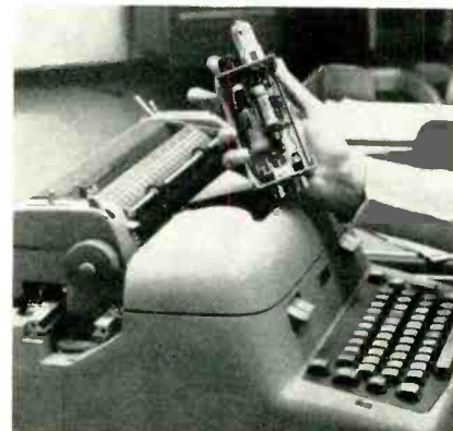
Electric typewriter with electronic tabulator control
