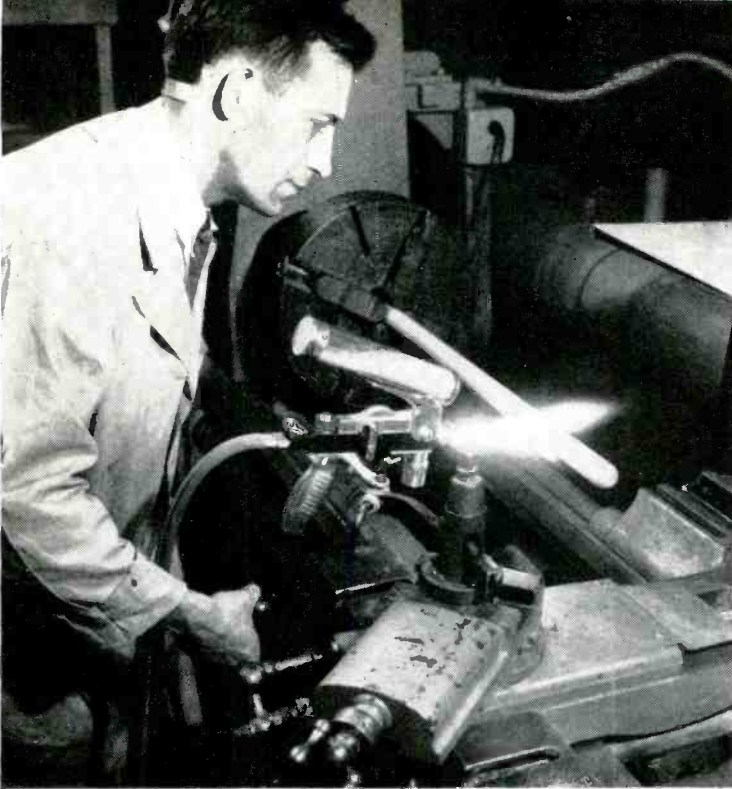
Flame-sprayed ceramic coating is applied to thermocouple tube using oxyacetylene equipment with special gun made by Metallizing Engineering
