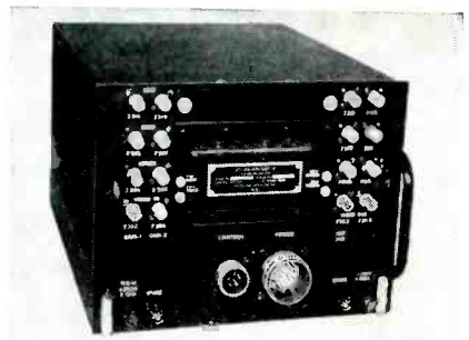
Video coder developed by Philco for the Air Force feeds information into transmitter (left)
