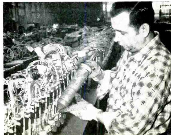
Sealing connectors for TM-61 Martin Matador tactical missile with synthetic rubber while fixtures and clips center wire leads
